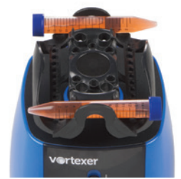
15 mL conical tubes x 2 (horizontally mounted)
