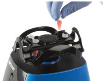
1.5/2 mL microfuge tubes x 4 (vertically mounted)
