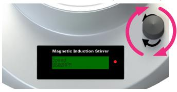
Once a program has started, the speed, cycle and time can be monitored. The stirring speed can be adjusted while a program is running.
